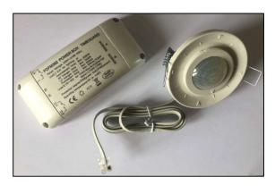
The sensor is a ceiling flush mount presence detector for indoor applications in commercial and domestic locations, and is supplied pre-wired, (approx. 1m long), which connects to the supplied Power Box, the power box requires securing above the finished ceiling.
