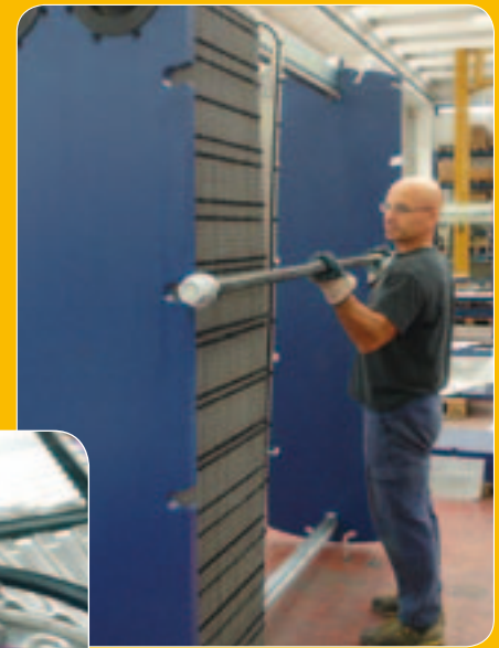
CIAT's patented "Plug-in" gaskets
