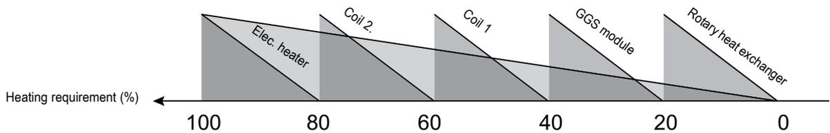
The order in which the various heat generators are activated can be configured. Coils available to meet the heating requirements
