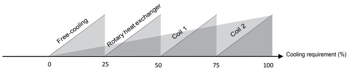
If coil 1 is configured as Mixed, the action on its valve will be limited to prevent a drift in the temperature for the return network to the heat pump.
