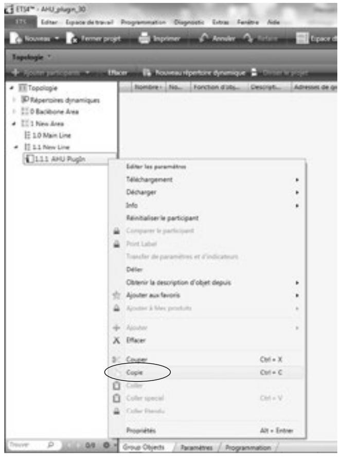
Open or create the final project for the system and right-click on the mouse to paste the CAREL plugin, once or more depending on the number of CAREL devices to be integrated. The address of each device is automatically incremented. If necessary, you can manually change the address of a device in Properties.
