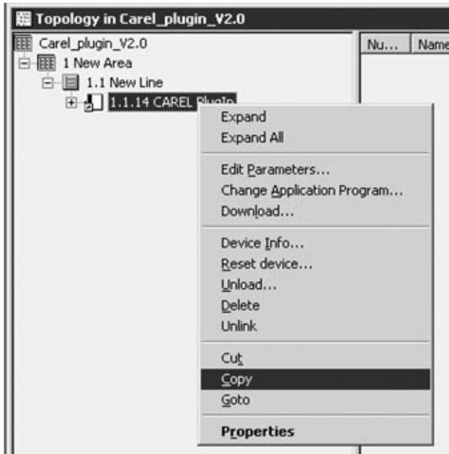
. Open or create the final project for the system and right-click on the mouse to paste the CAREL plugin, once or more according to the number of CAREL devices to be integrated. The address of each device is automatically incremented. If necessary, you can manually change the address of a device in Properties.
