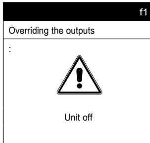
If all the controller's outputs are overridden, the alarms will not be signalled on the door of the electrical box or on the display. Disconnecting the display will maintain the override and may result in damage to the hardware.
