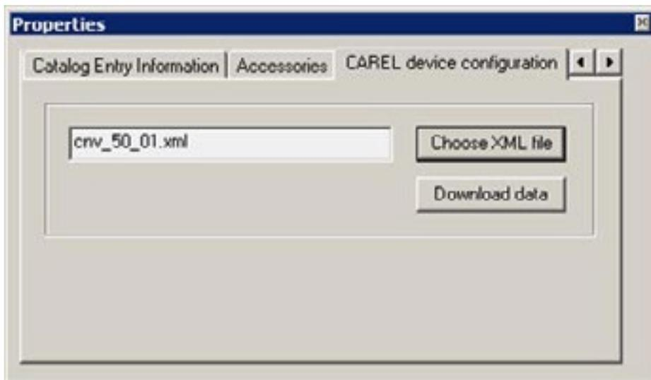
Use "Choose XML file" to open the XML configuration file required.
