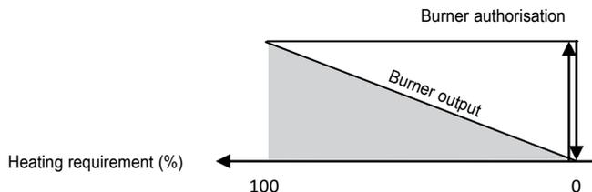
If ramp up/down start is selected, the burner output will increase or decrease gradually based on the difference between the heating requirement and the burner output. Depending on this difference, every second, there will be an action corresponding to the following value: addition or deletion of 100/ramp time.
