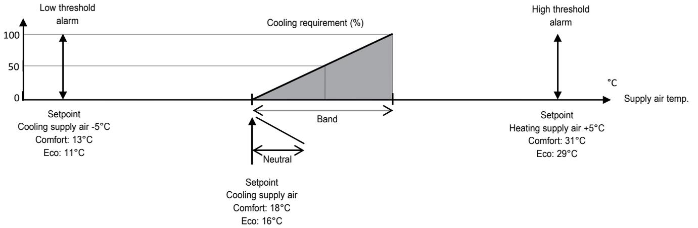
→ When the temperature drops, the controller will calculate the heat requirement needed to keep this temperature constant. It will gradually adjust the output of the 5 controllable heat generators:
