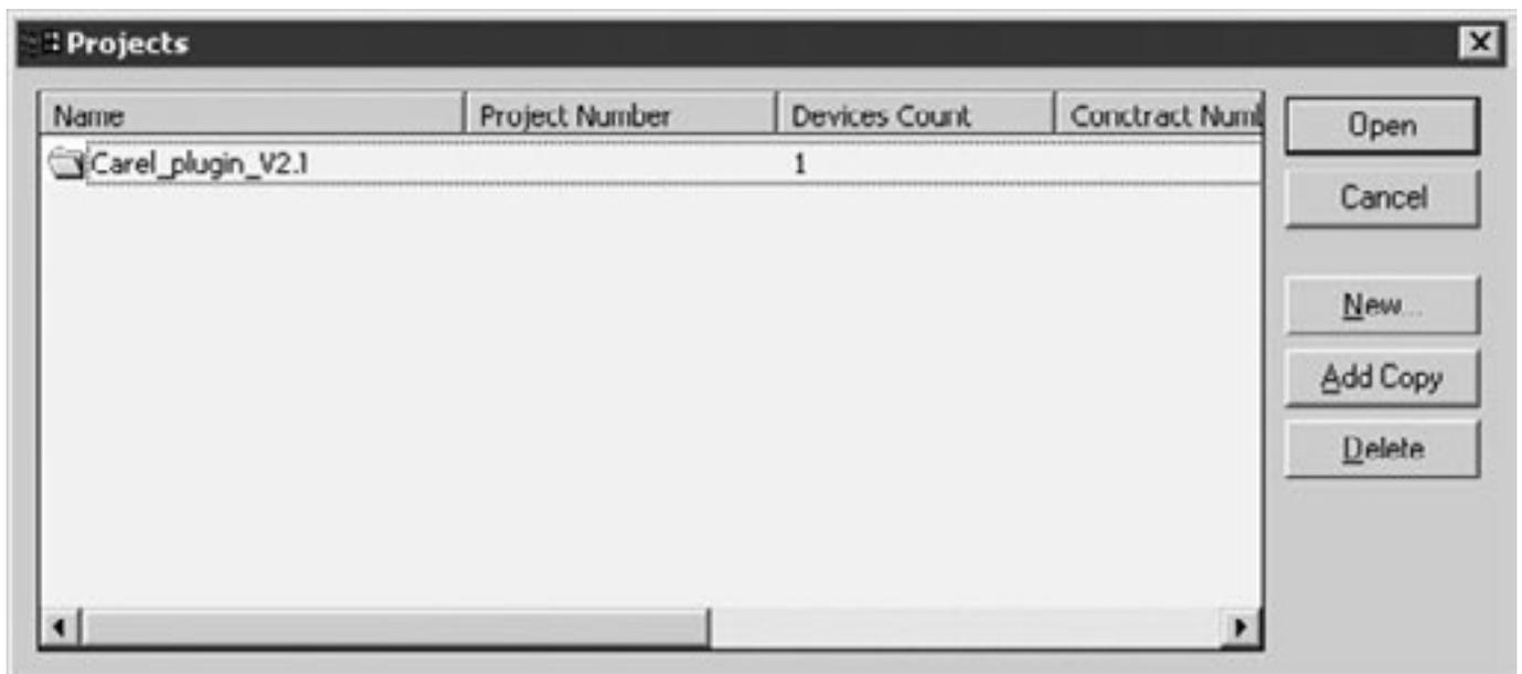
. Open the project using Open, select the device "CAREL Plugin", right-click on the mouse and select Copy:
