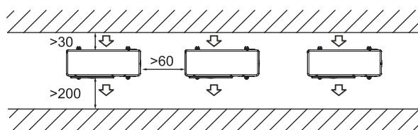
Parallel connect the front with rear sides. unit:cm
