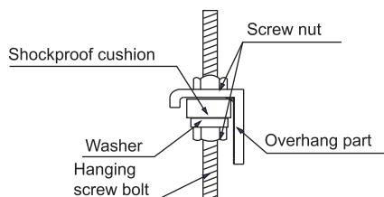
2.3.3 Screw the nuts to suspend the unit
