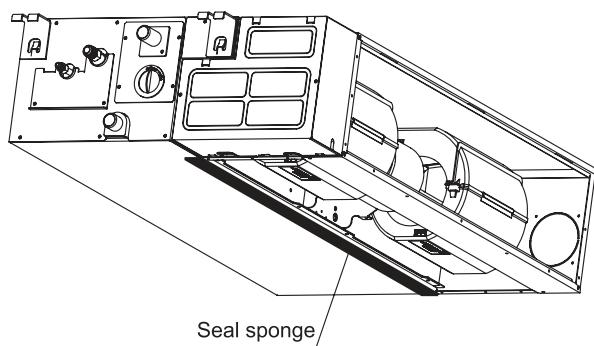
3. Attach the air filter to the flange in the manner shown in the diagram.
