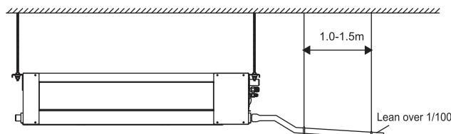
For unit with the drain pump
